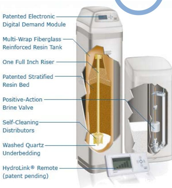
**Cross sectional view of an EcoWater Systems water softener**
